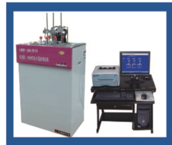
Vicat temperature tester of softening point
